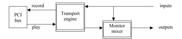
The arrows labeled "record" and "play" are the pipes – data moving over the PCI bus.
